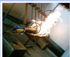
Fire Rated cable Fire Demo Test. Results show that the wires can last for at least 3 hours.
