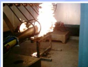
Fire Rated cable Fire Demo Test. Results show that the wires can last for at least 3 hours.
